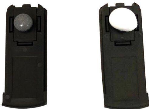
Figure 3: Images showing the lamination adhesives before (left) and after (right) curing.
